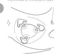
Turn inside out the silicone mask Be sure that the electrodes of the silicone mask and controllers are aligned.
