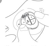
Align attachment guideline marks on the controller and the silicone mask Then insert a corner of the controlle into a chase of the silicone mask.
