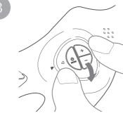
Hold an edge of the controller with your thumb and squeeze the controller into underneath of the mask to set it firm. Set the other controller following the same steps described above.
